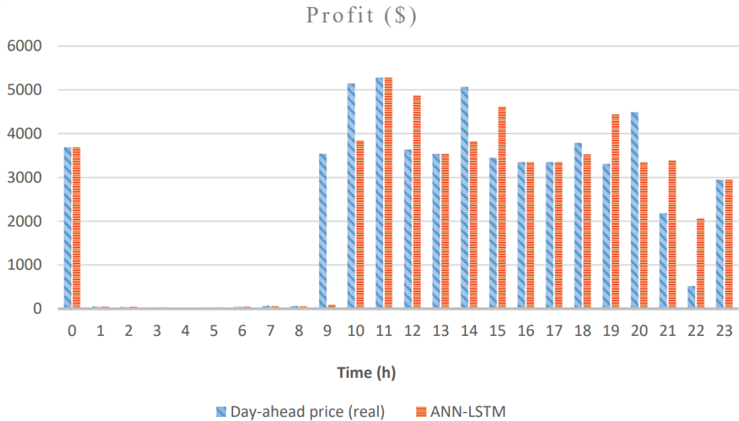
Figure 4.5 : Profit of ANN-LSTM model and ex-post day-ahead prices according to the hours of the day on 14 November.
