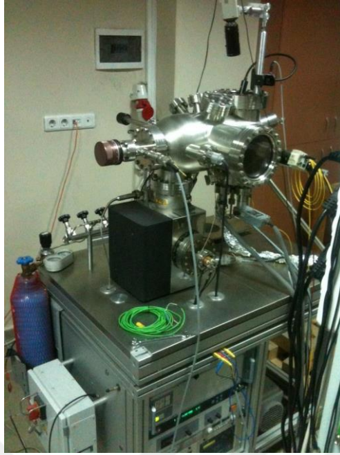
Figure 2.10 : AFM/STM in Ultra High Vacuum.
