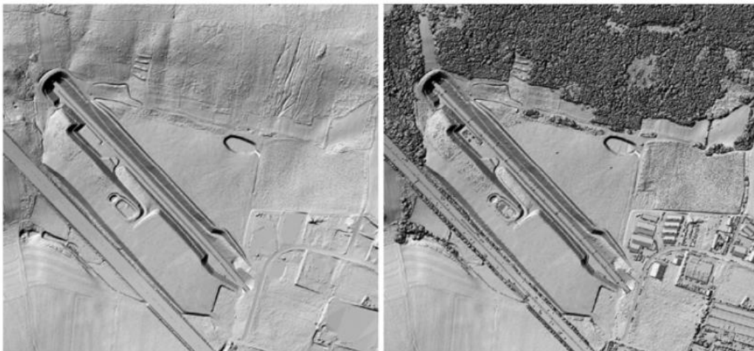
Figure 5.3 : The difference between DTM (left) and DSM (right) (Elste, 2018).
