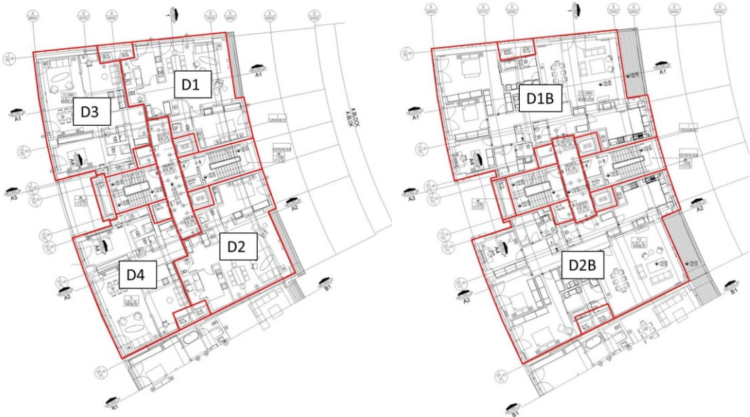
Figure 5.2 : The thermal zone areas on architectural plan of A Block.
