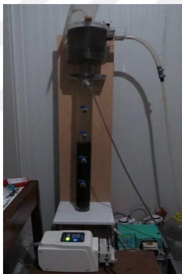
Figure 4.8 : EGSB reactor No.1, actual set up used with fresh urine.
