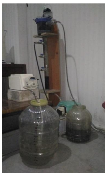
Figure 4.10 : EGSB reactor No.2, actual set up used with stored urine.
