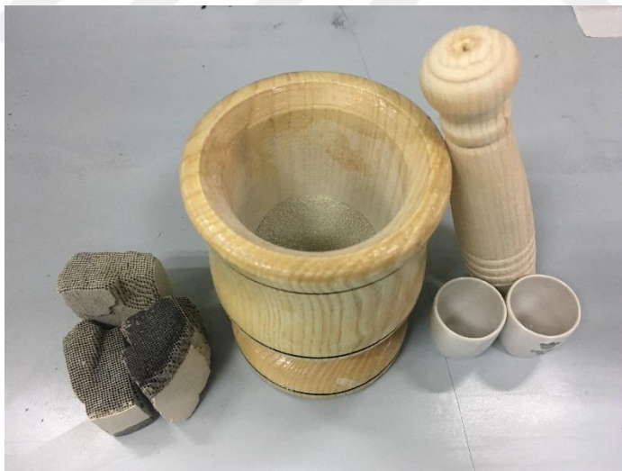
Figure 3.2: Spent catalyst before and after grinding.
