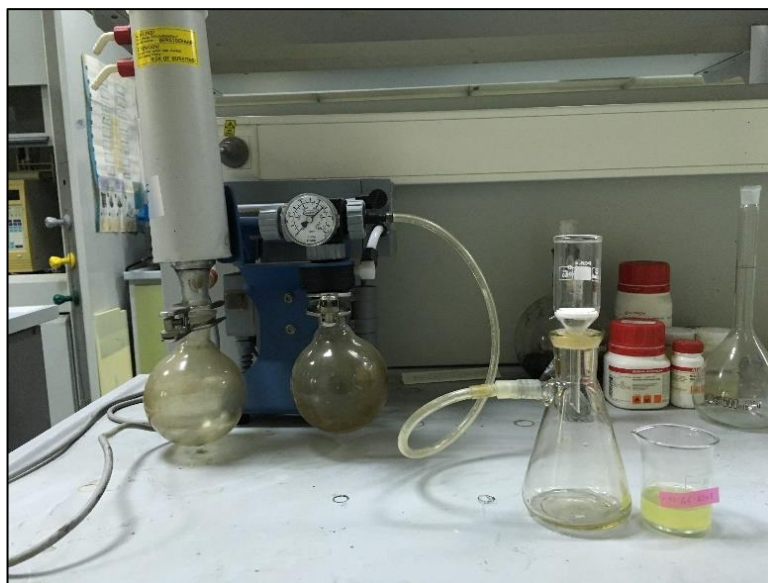
Figure 4.4: Filtering the residues with vacuum pump is required.
