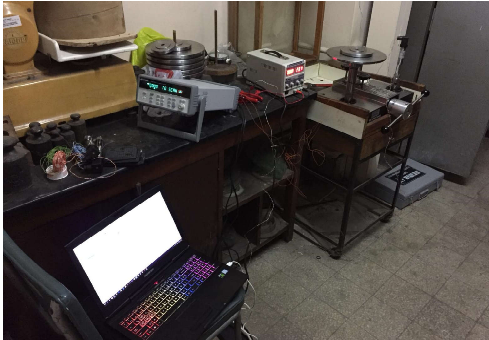
Figure A.2 : Pressure calibration with dead-weight pressure tester.
