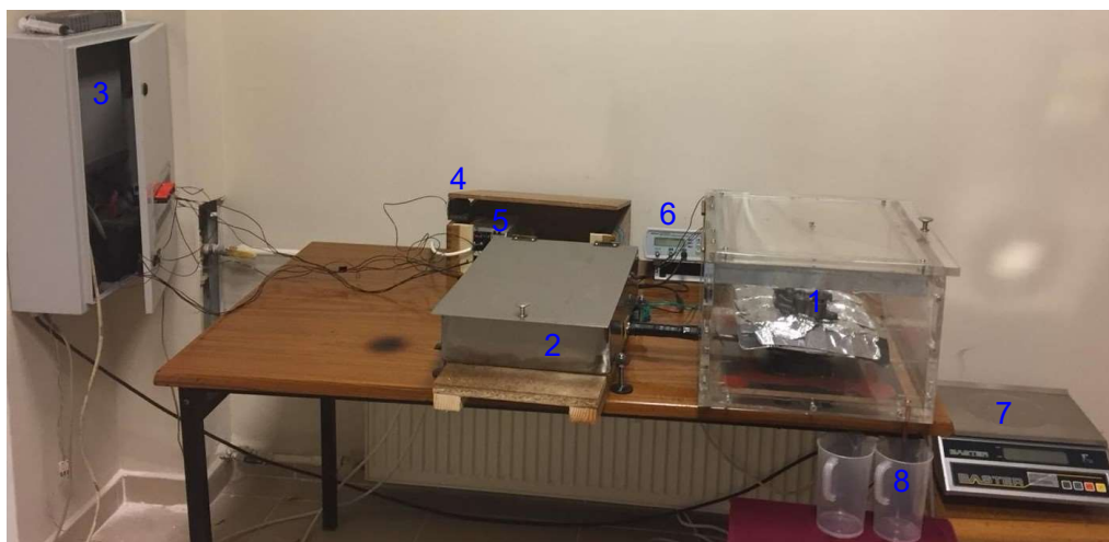
Figure 2.33 : Instruments of the experimental set up: 1. CIC 2. Pre-heated oil sump 3. Control panel 4. PID controller 5. Direct current relay 6. Frequency generator 7. Precision balance 8. Beakers
