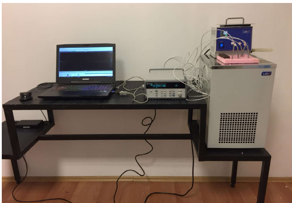
Figure A.1 : Temperature calibration with calibration bath.
