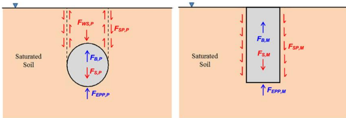
Figure 2.6 : Schematic of forces acting on pipeline (left) and manhole (right) (Chian & Tokimatsu.2012).
