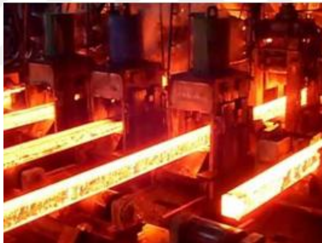
Figure 2.5: Strand casting method of steel manufacturing [12].
