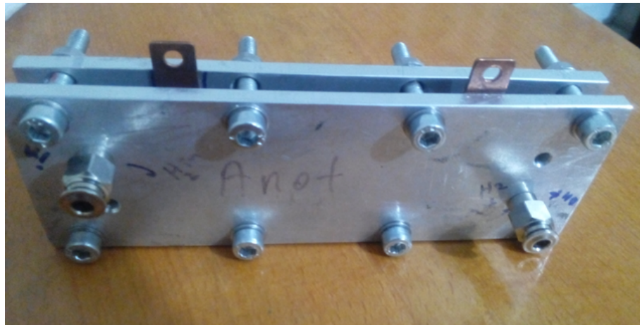
FIGURE 2.14: Single cell Assembly without air blower
