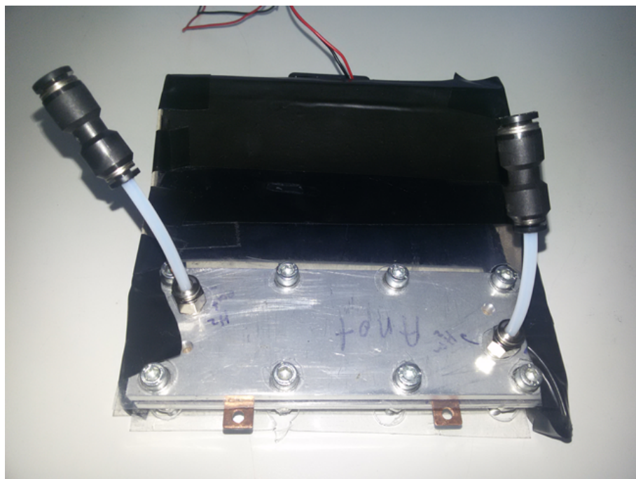
FIGURE 2.15: Single cell Assembly with air blower
