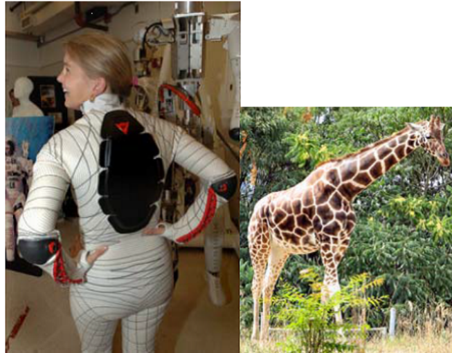
FIGURE 2.29: The ultra maneuverable and lightweight space suit, partially inspired by the tight skin of a giraffe's legs, which helps to regulate blood pressure. It relies on mechanical pressure rather than gas pressure to support human life in a thin atmospheric environment such as Mars
