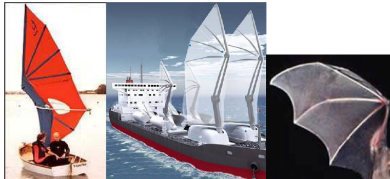
FIGURE 2.28: The sails of this cargo ship are designed based on an analogy to a bat's wing.
