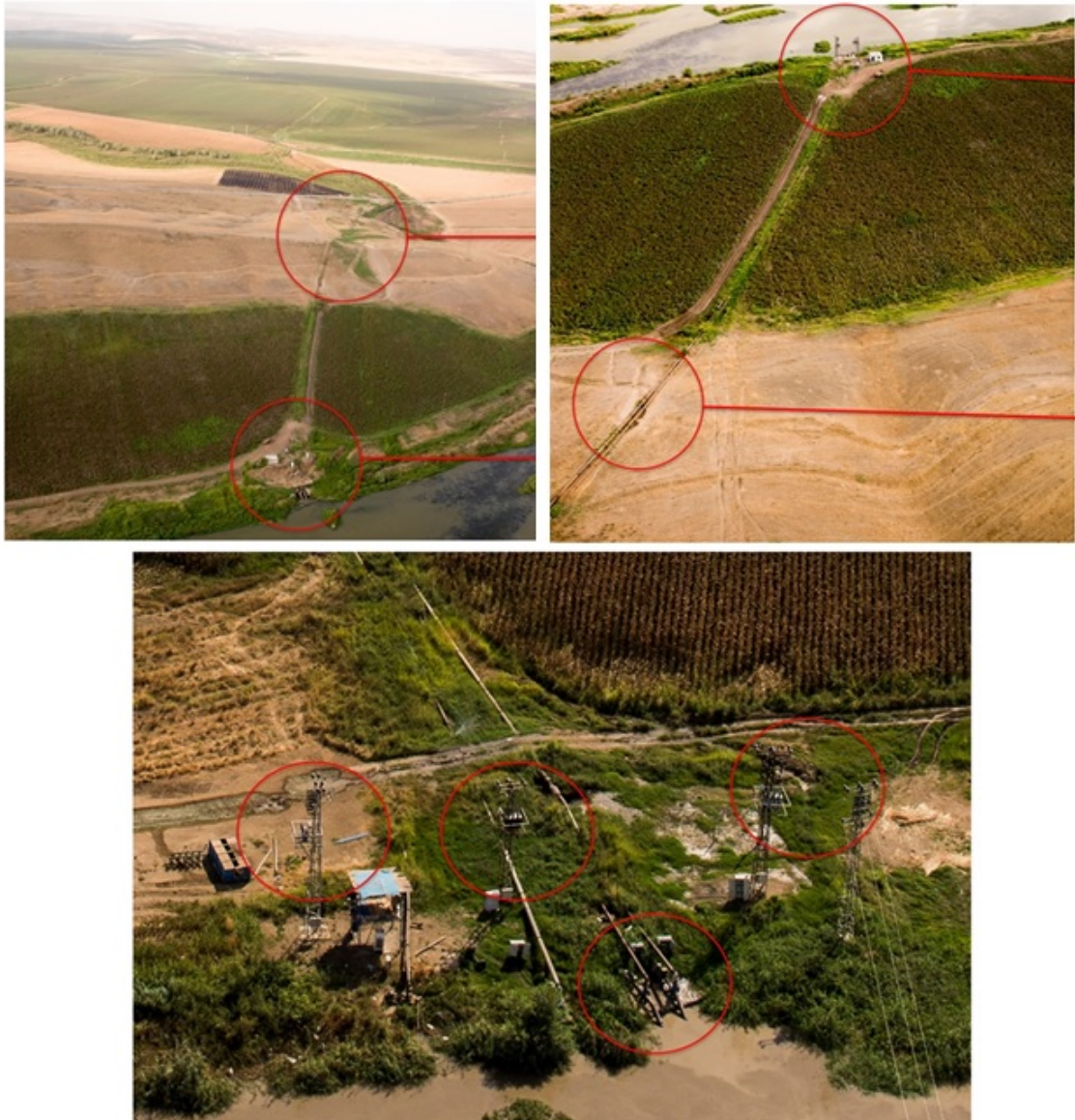
Figure 3.5: Illegal electricity use for agricultural irrigation for pumping water to ground and transporting on the ground
