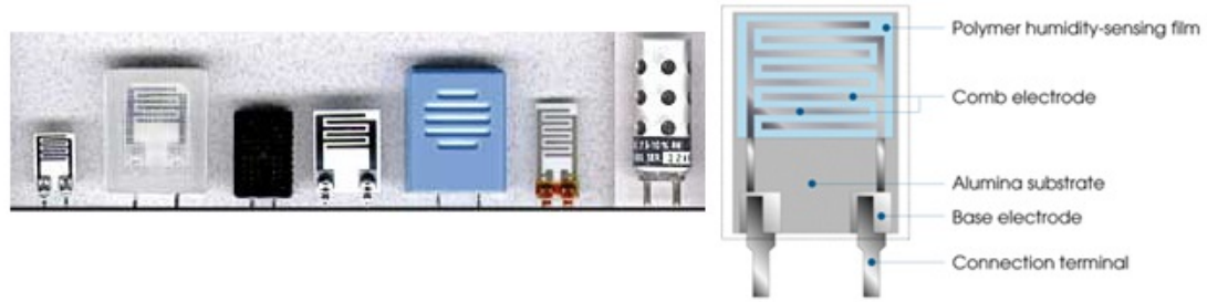
FIGURE 1.3: Basic structure of resistive type humidity sensor
