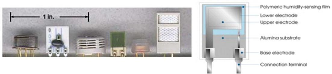
FIGURE 1.2: Basic structure of capacitive type humidity sensor [10]
