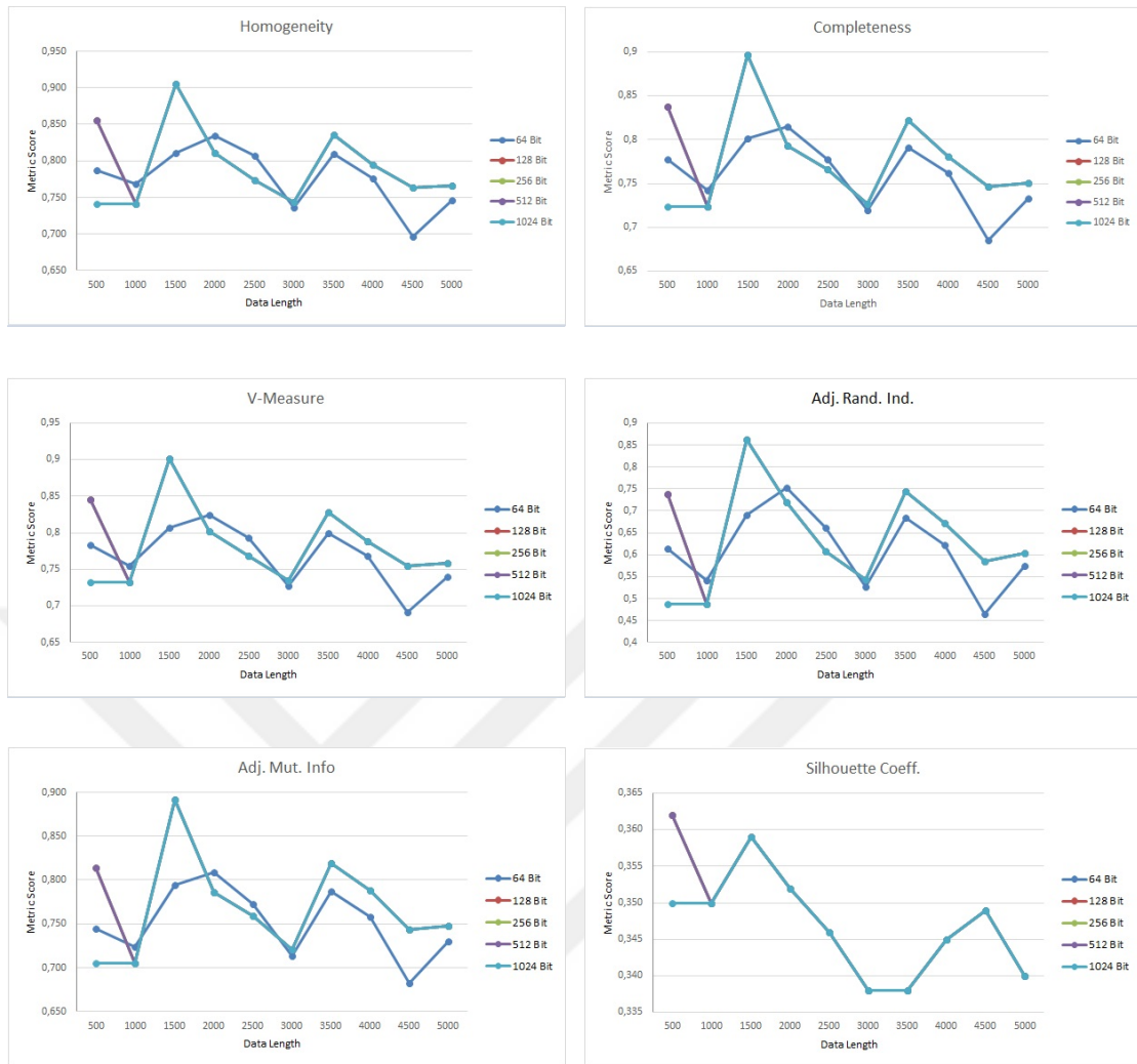
FIGURE 5.51: Charts that show change of each evaluation metrics score by data length for different key lengths and for K-Means Algorithm
