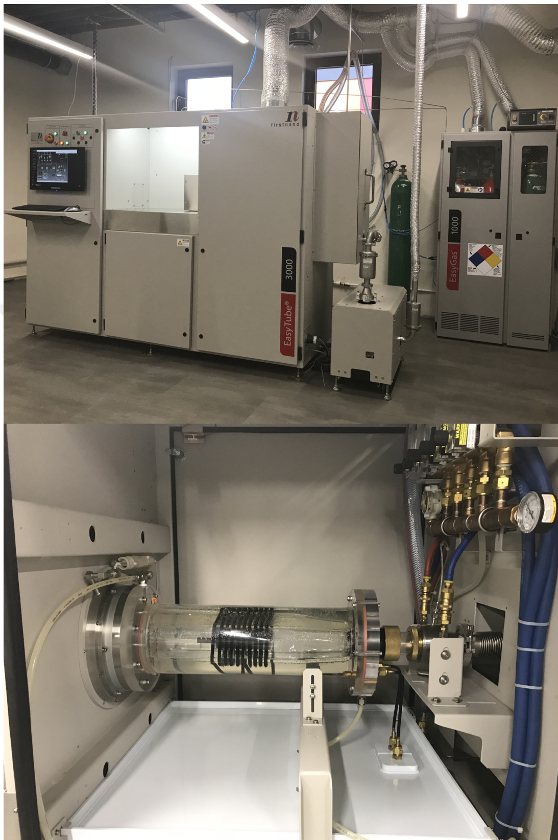
FIGURE 2.1: MOCVD equipment used for the growth of the nanowires. The lower image depicts the quartz tube inside where the reaction occurs.
