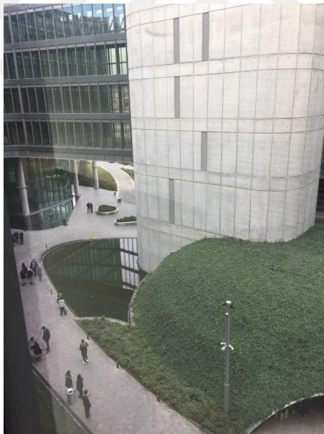
Figure 3.21 Extensive green roof - Garanti bank tech campus
