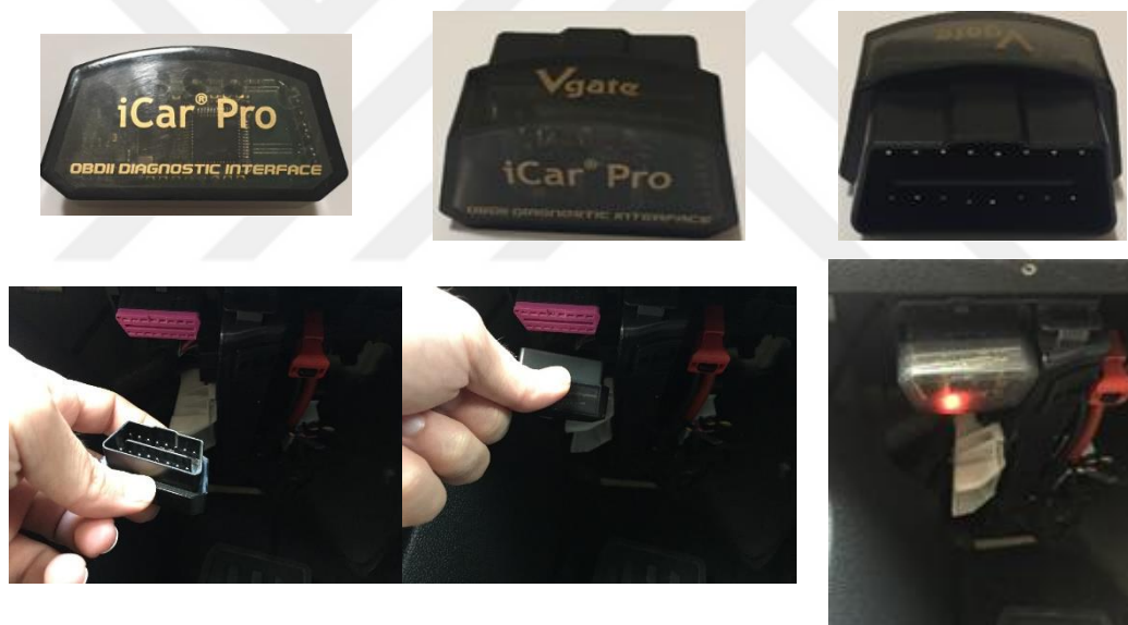
Fig. 4.48. OBD II diagnostic interface
