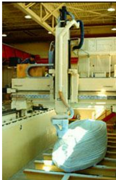
Figure 136: Physical model of object constructed from computer model with numerically controlled machine.
