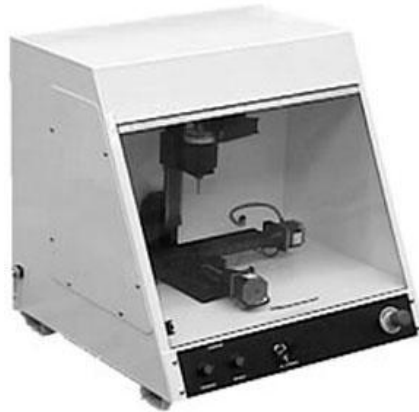
Figure 141: Denford Micromill 2000 desktop milling machine, (Seely, Jennifer C.K. and Sass, Larry. 2004)
