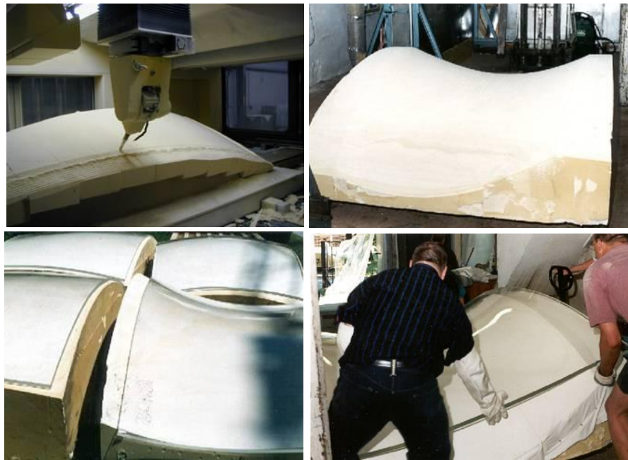
Figure 221: Cutting the shell pieces of the exterior cover. (Source: http://lapa.epfl.ch/downloads/programming_as_design_method.ppt .)
