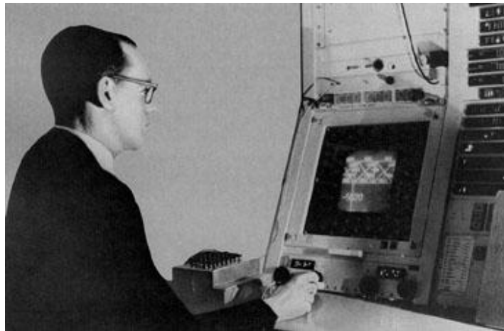
Figure 4: Ivan Sutherland at the console of the MIT TX-1 demonstrating his PhD dissertation software Sketchpad in 1963. source MIT (Source: http://accad.osu.edu/~waynec/history/lesson2.html )
