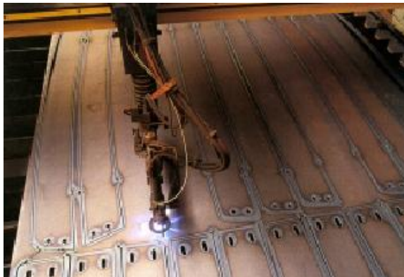
Figure 204: Plasma-arc CNC cutting machines for cutting the pieces,(Marc Aurel Schnabel, 2003)
