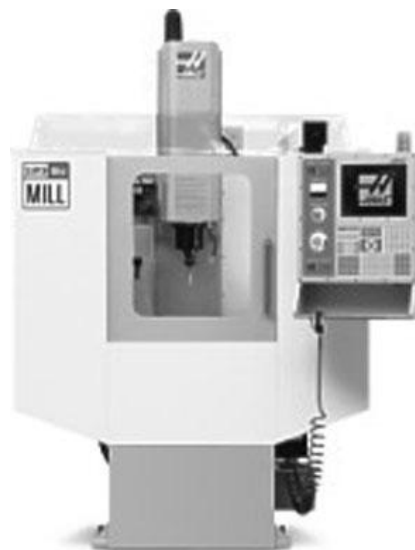
Figure 142: HAAS Super Mini Mill, (Seely, Jennifer C.K. and Sass, Larry. 2004)
