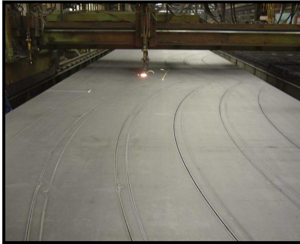
Figure 233: Using the digital machines for cutting the edges of the wire frames pieces.
