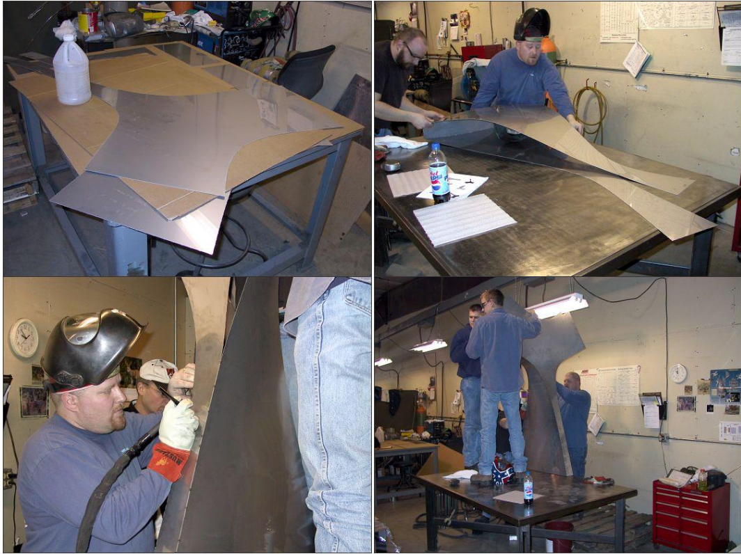
Figure 174: The waterjet cutter was used for cutting stainless steel parts, then the staff starting welding the parts
