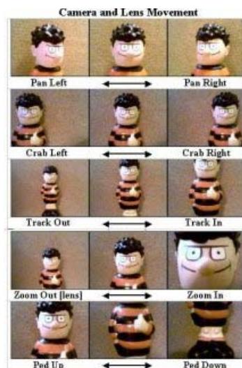
Figure 2.1: Graphical definition of camera motion
