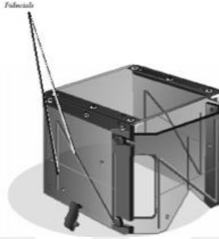
1) MRI indicator box 2) MR indicator box fiducials 3) CT indicator box
