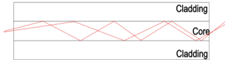
Figure 2.9. Schematics of step index multi mode fiber
