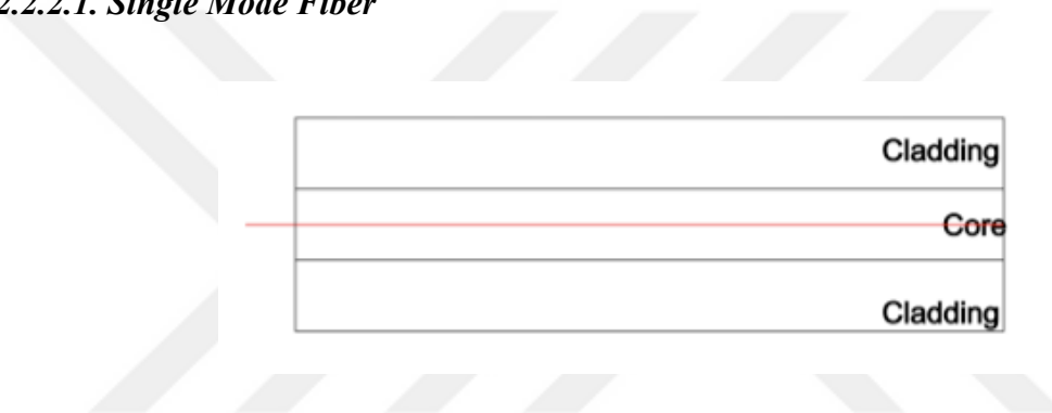
Figure 2.8. Schematics of single mode fiber
