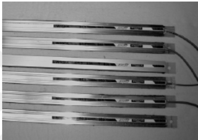
Figure 1.3. Fiber-optic strain gauge
