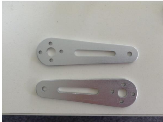
Figure 3.2.10. The servo extensions, after sanding and galvanization.
