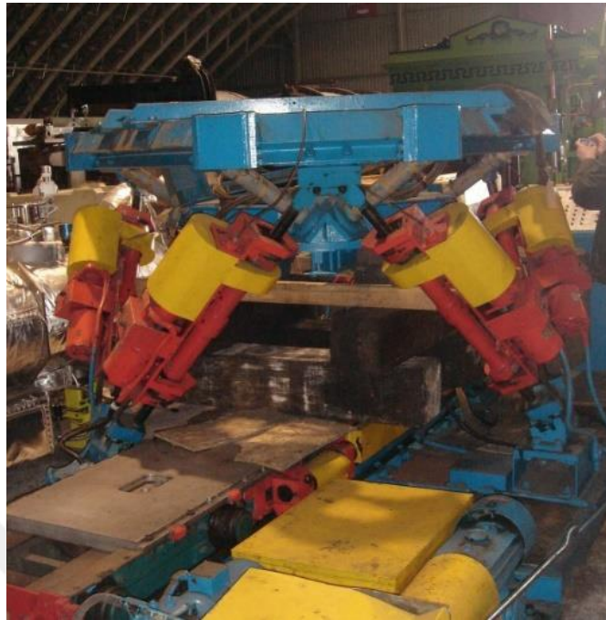
Figure 1.2. Tire Testing Machine by Eric Gough, as a Stewart Platform [2]
