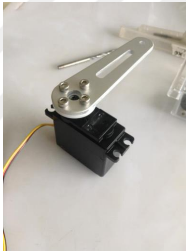
Figure 3.2.11. One of the servos with its extension assembled.
