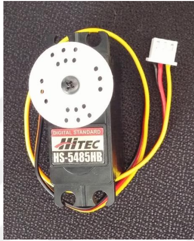
Figure 3.3.1. Servo Motor – HITEC HS-5485HB
