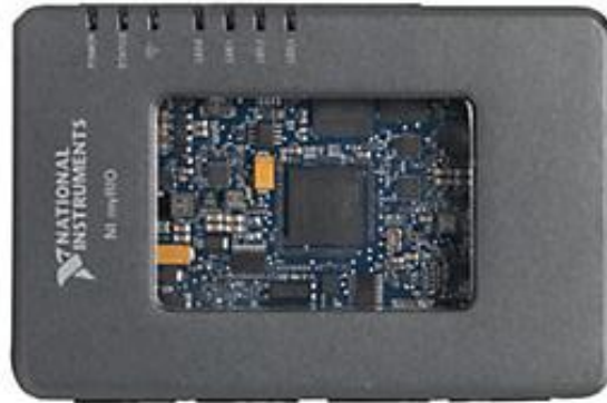
Figure 3.3.3. myRIO microprocessor for controlling the system [8]
