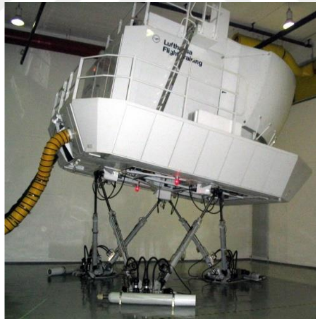
Figure 1.1. A Flight Simulator as Stewart Platform [1]
