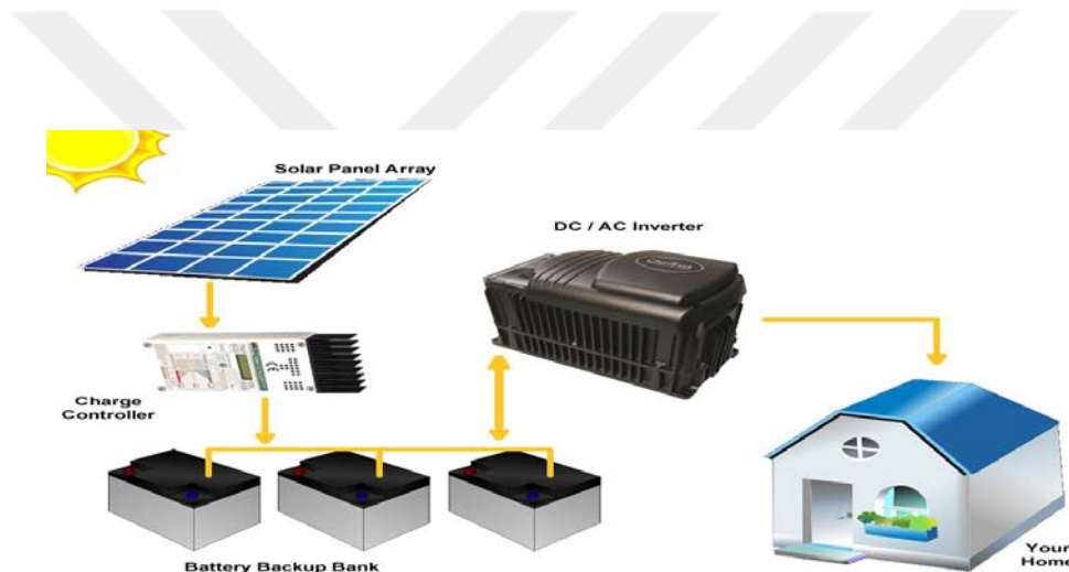
Figure 3.1: Basic diagram for photovoltaic installation
