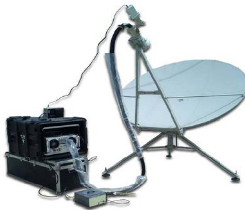
Figure 1.7: Satellite HPA, LNB and Antenna
