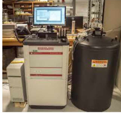
Şekil 3.4. Quantum Design PPMS-9t titreşimli örnek magnetometresi (vibrating sample magnetometre, VSM)
