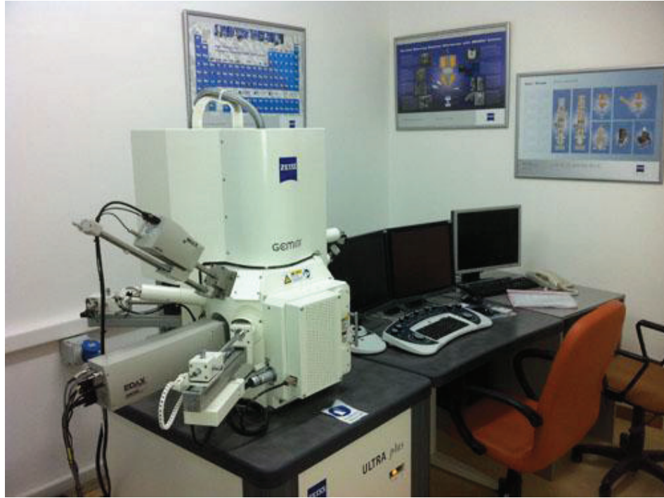
Figure 2.6 Ultra plus high resolution field emission-scanning electron microscope
