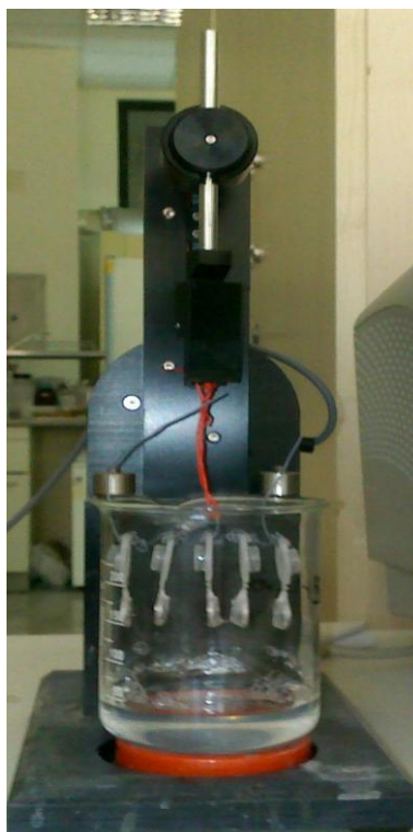
Figure 2.2 : Typical dip coating machine used in all experiments.
