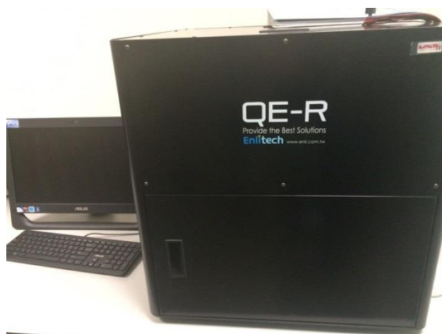
Figure 3-23: IPCE (EQE) measurement system.
