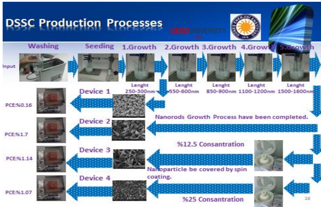
Figure 4-13: The Production Phase of the Each Devices and Comparison of the Efficiency
