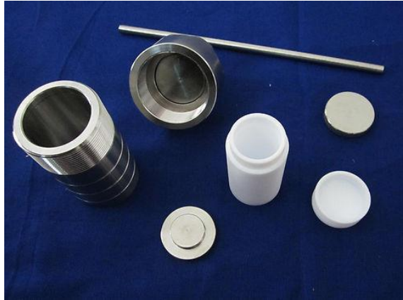
Figure 2-15: Teflon Pot Which is Used in The Hydrothermal Method [111] .
