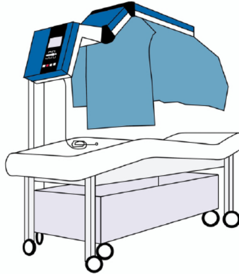
Figure 3.7 Schematic drawing of the Iratherm system for whole-body hyperthermia (Wust et al., 2002).
