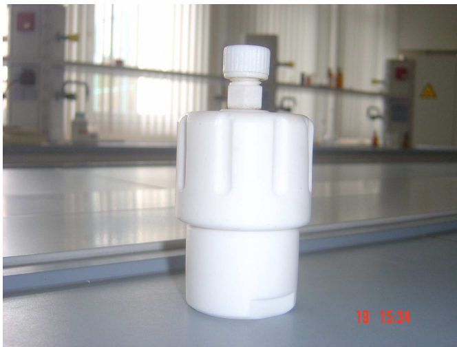
Figure 1.5 Autoclave used in hydrothermal process.
