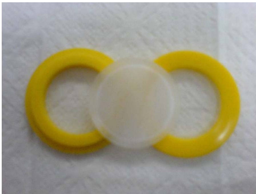
Figure 4.2 Teflon PTFE filter and rings (The image was taken in our lab).
