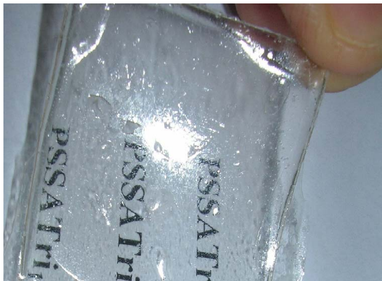
Figure 5.3. Photograph of PSSATri x film with a thickness ca. 200 \mu\text{m} .
