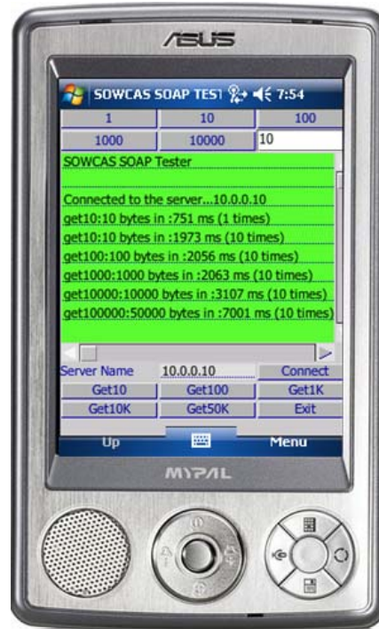
Figure 5.1 The performance testing program GUI on ASUS Pocket PC.
