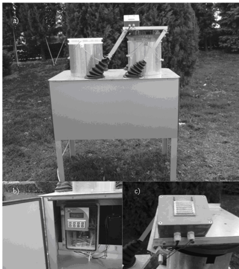
Figure 2.2 a) Our homemade type Wet/Dry Rain sampler, b) PLC digital information part c) Rain sensor.
