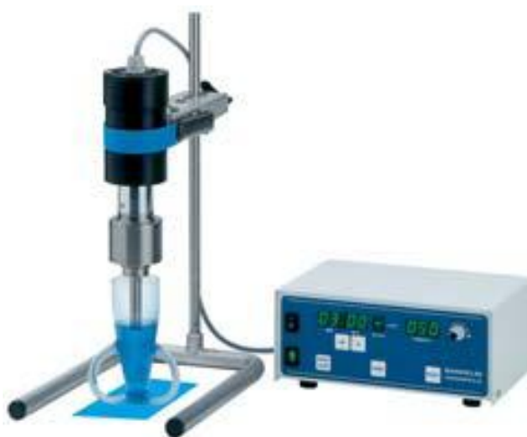
Figure 2.3 The ultrasonic homogenizer for used sonochemical synthesis.
