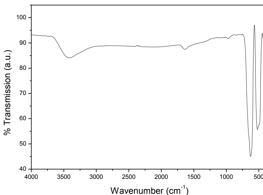
Figure 3.40 FTIR spectrum of as-synthesized \text{Mn}_3\text{O}_4 NPs.
