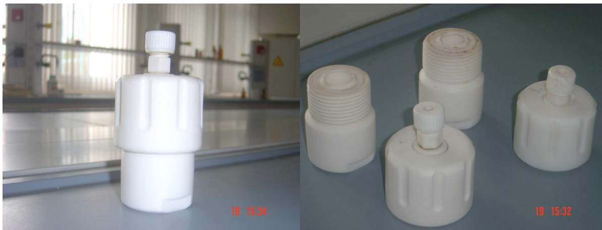
Figure 2.1 Autoclaves used for hydrothermal synthesis.
