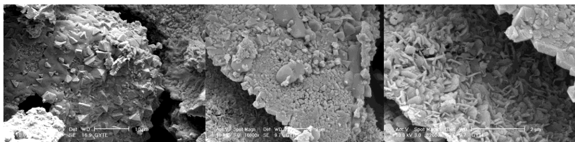
Figure 3.77 SEM micrographs of \text{Co}_3\text{O}_4 NPs powder at different magnifications obtained after calcination of the dried gel precursor at 800 °C for 3 h.
