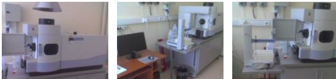
Figure4.6 Induction Combined Plasma (ICP)
