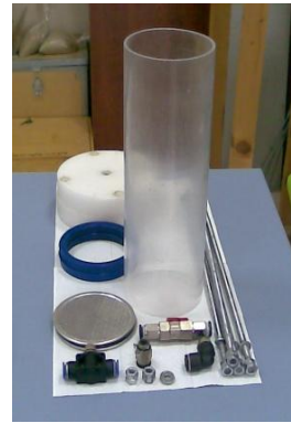
Figure 4.5 Parts of the Column Cell
