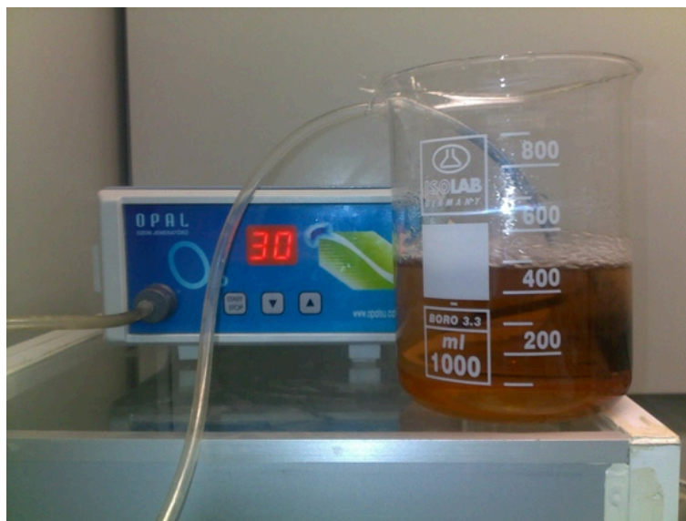
Figure 3.2 The picture of the Ozone Generator
