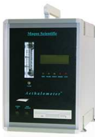
Figure 2.14 The Portable Aethalometer Model AE 42 (Magee Scientific, 2010)
