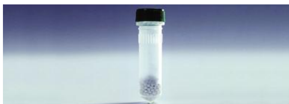
Figure 2.1 MagNA Lyser sample tube: 2 ml screw-cap tube prefilled with 1.4 mm ceramic beads used for homogenization of tissue samples.
