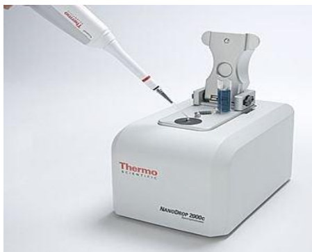
Figure 2.3 Thermo nanodrop device: Usage for spectrophotometric measurement of isolated RNA quantity and purity.
