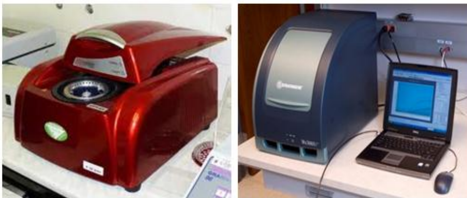
Figure 2.7 RT PCR devices: First is “Rotor-Gene 6000 (Corbett)” for x36 samples and second is “Stratagene MX3000p” for x96 well plate.
