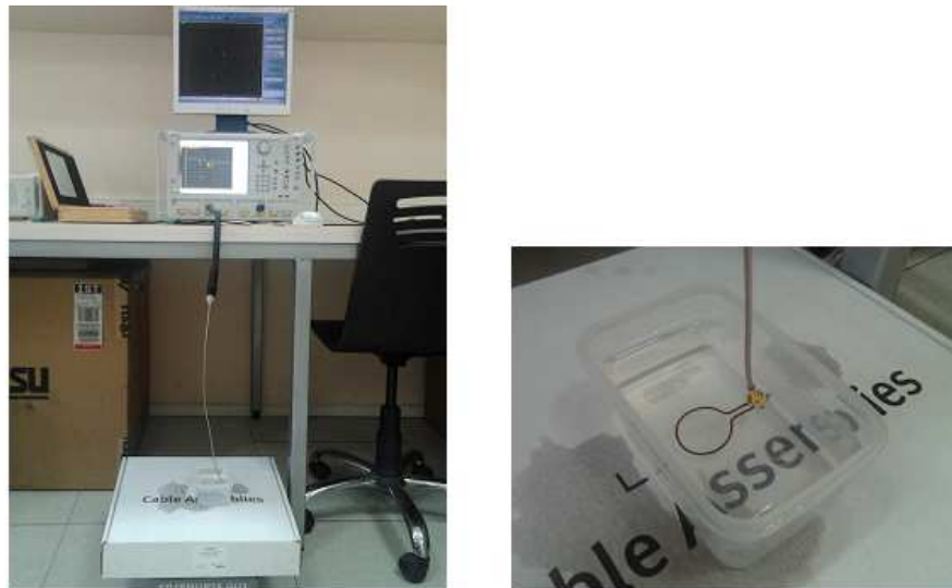
Figure 4.28 Measurement setup for return loss measurements.
