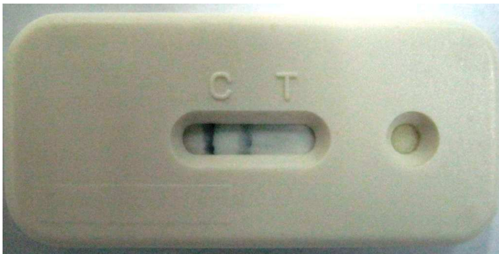
Figure 4.27 LFTS showing the test line and the control line.
