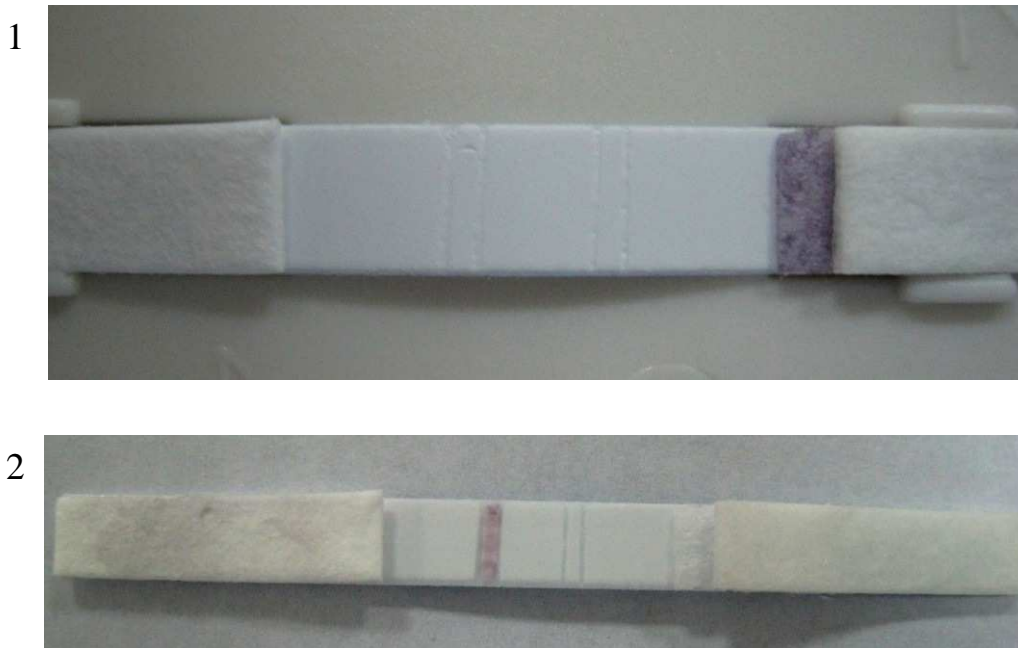
Figure 4.24 An indented line was made on the membrane (1). A red color was seen on this line where the capture reagent was immobilized (2).
