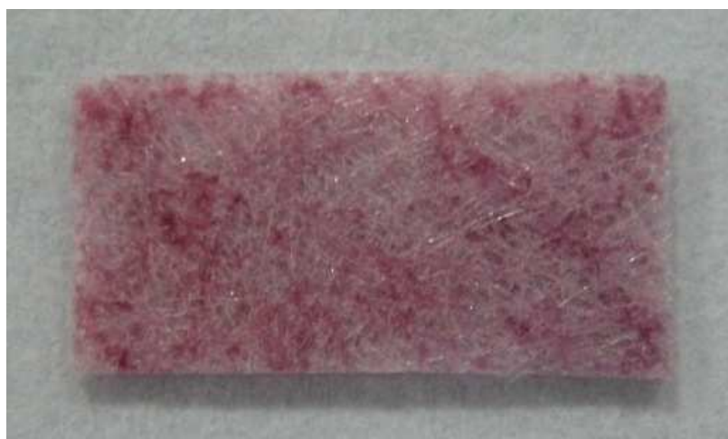
Figure 4.17 Conjugate pad showing even distribution of the gold labeled McAbs into the pad.
