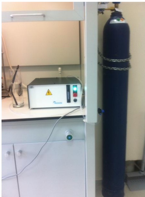
Figure 3.2 The picture of the Ozone Generator.
