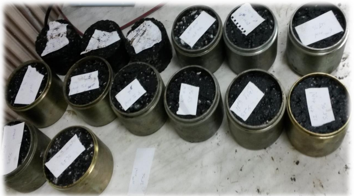
Figure ( 5 ) agroup standard marshal specimen of hot mix asphalt produced for testing
