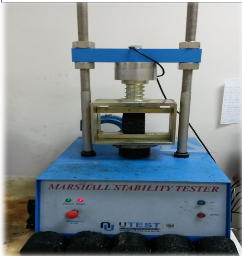
Figure (18) shows indirect tensile test apparatus
