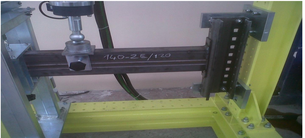
Setup for Beam End Connector Bending Test According to the European Standard (European Committee for Standardization, 2009)
