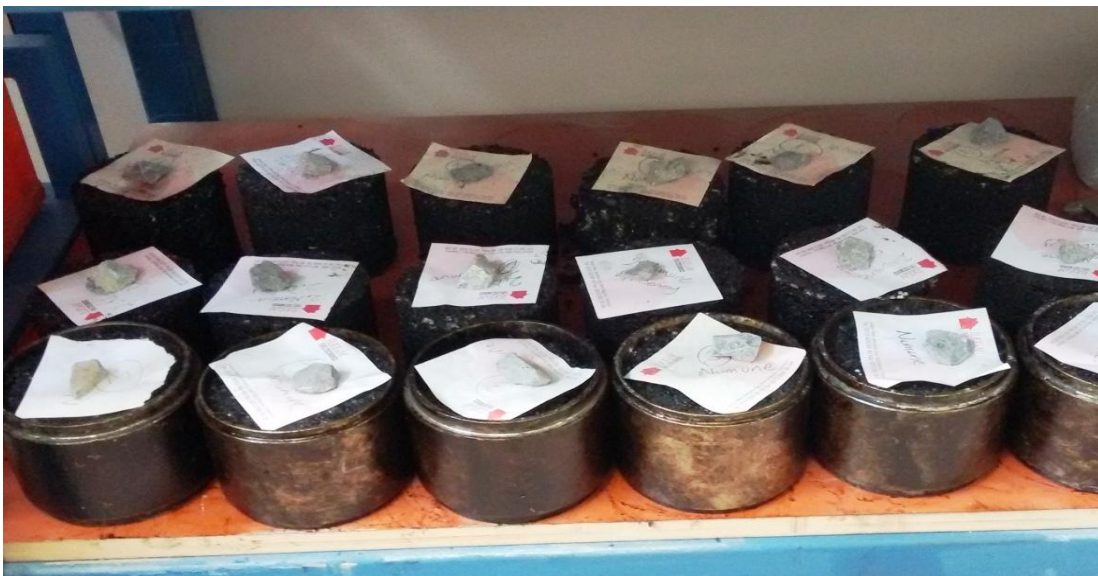
Figure 3.7 Standard Marshall Samples Prepared For Testing.
