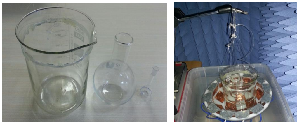
Figure 6.6 Different beakers used during the measurements and placement into the applicator.
