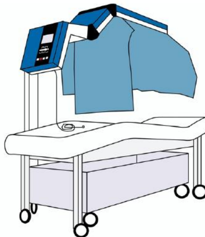
Figure 2.7 Schematic drawing of the Iratherm system for whole-body hyperthermia (Wust et al., 2002).
