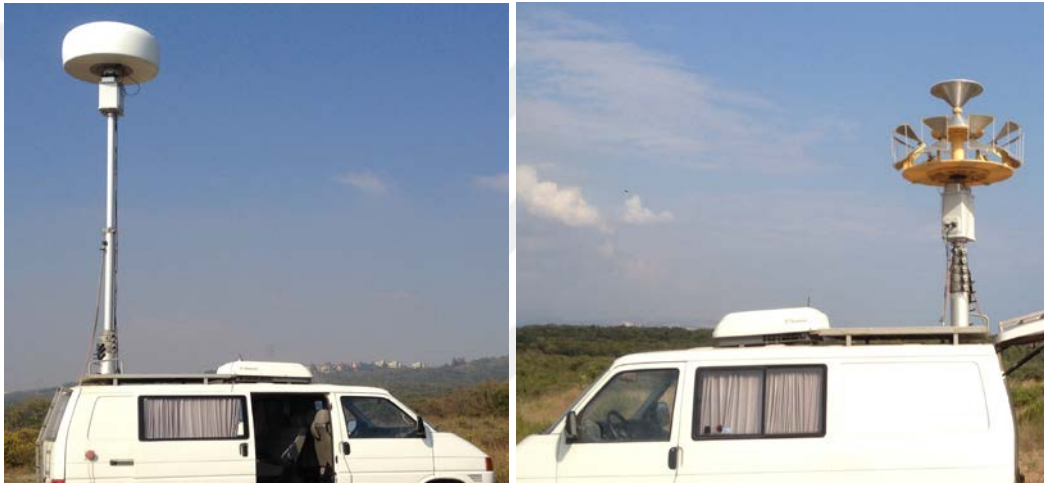
Figure 4.6 DF Antenna System a) DF-A0029 at The Top of The Vehicle b) in a Field at The Top of The Vehicle.
