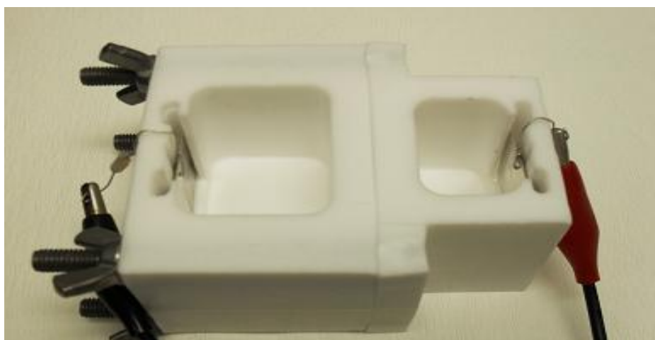
Figure 3.1 Experimental set-up of double tank cell.
