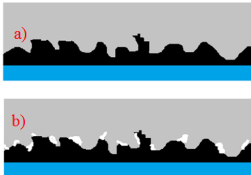
Figure 5.7 Result of coatings a) Slow coating of Al b) Fast coating of Al [51].
